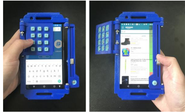
Figure 1. Interactiles allows people with visual impairments to interact with mobile touchscreen phones using physical attachments, including a number pad (left) and a multi-purpose physical scrollbar (right).
