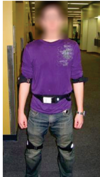
Figure 1: The placement of the Microleap2 devices.
