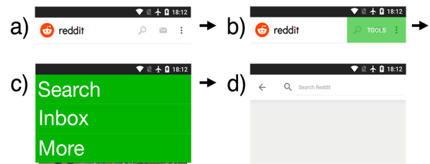
Figure 4. This interaction proxy replaces one interaction with a sequence of two interactions. (a) An interface contains several small adjacent targets. (b) Replaced with a single larger “Tools” button. (c) Selection displays a menu of the original targets. (d) A selected item is activated.
